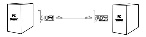
Connecting two computers simply requires each computer to have a Network Card, such as the Belkin Notebook Network Card for laptop computers, or the Belkin Desktop Network Card for notebook computers. Simply connect the two Network Cards using a crossover Ethernet patch cable, such as Belkin part number:
